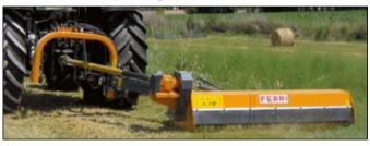
The gearbox position located outside of the transmission cover allows greater off-set of the flail head reducing the Pto shaft angle in work.
