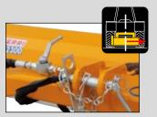
Hydraulic block tap side movements for transport with manual activation (no chains or holders).
