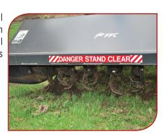
Scarifier assembly increases productivity by combining the tractive effort and force of the loader with the hydraulic horse power of the tiller
