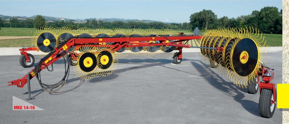
Inorder to adapt to extreme field conditions, hay rakes must be solid and sturdy. This is why the drawbar and the rake wings have been made using a large lattice framework of structural tubing to make them tough and fully reliable over time, however hard they are made to work. Despite their size, these machines are easy to handle and transport and very user-friendly.
