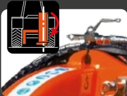
Hydraulic block tap for transport with manual activation (no chains or holders).
