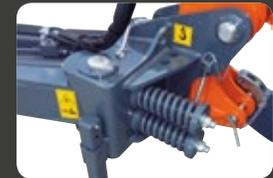
Shock absorber with mechanical springs.
