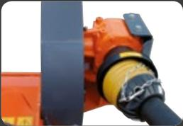
Gearbox is fitted outside the transmission cover.
