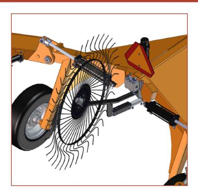
Pequea's kicker wheel option is designed to move the hay that lies below the center of the rake and does not get touched by the two main rake beams. The kicker wheel is used to prevent moisture from become trapped in this hay. The kicker wheel itself is hydraulically controlled and the cylinder is installed with just two hoses that connect directly to the manifold.
