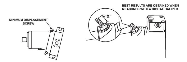
NOTE: These mulchers include a 6mm allen wrench and 19mm wrench to adjust the displacement screws.
