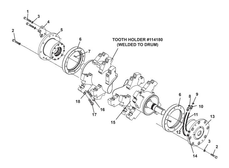
3-LINE - SKID STEER LOADER ASSEMBLY - #115630 5-LINE - SKID STEER LOADER ASSEMBLY - #115631 ROTOR ASSEMBLY
