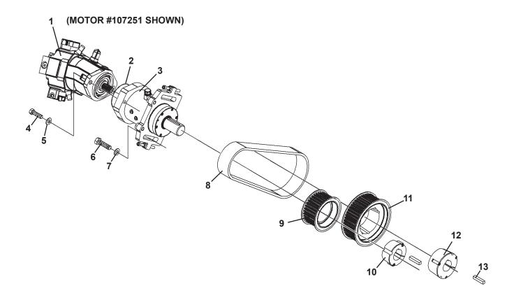
3-LINE - SKID STEER LOADER ASSEMBLY - #115622 5-LINE - SKID STEER LOADER ASSEMBLY - #115623 MOTOR AND DRIVE ASSEMBLY
