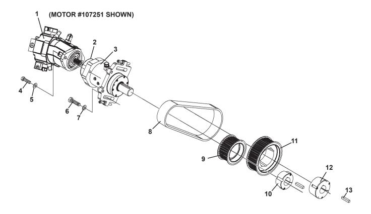
3-LINE - SKID STEER LOADER ASSEMBLY - #115630 5-LINE - SKID STEER LOADER ASSEMBLY - #115631 MOTOR AND DRIVE ASSEMBLY
