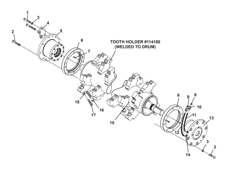
3-LINE - SKID STEER LOADER ASSEMBLY - #115622 5-LINE - SKID STEER LOADER ASSEMBLY - #115623 ROTOR ASSEMBLY
