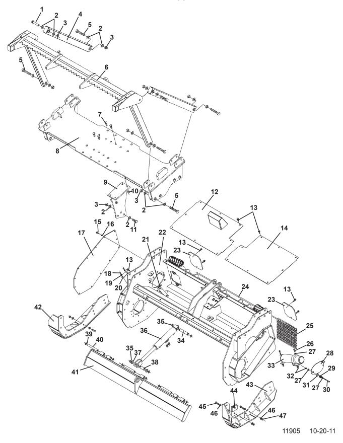
3-LINE COMBO (SKID STEER LOADER AND EXCAVATOR) ASSEMBLY - #115625 MAINFRAME ASSEMBLY
