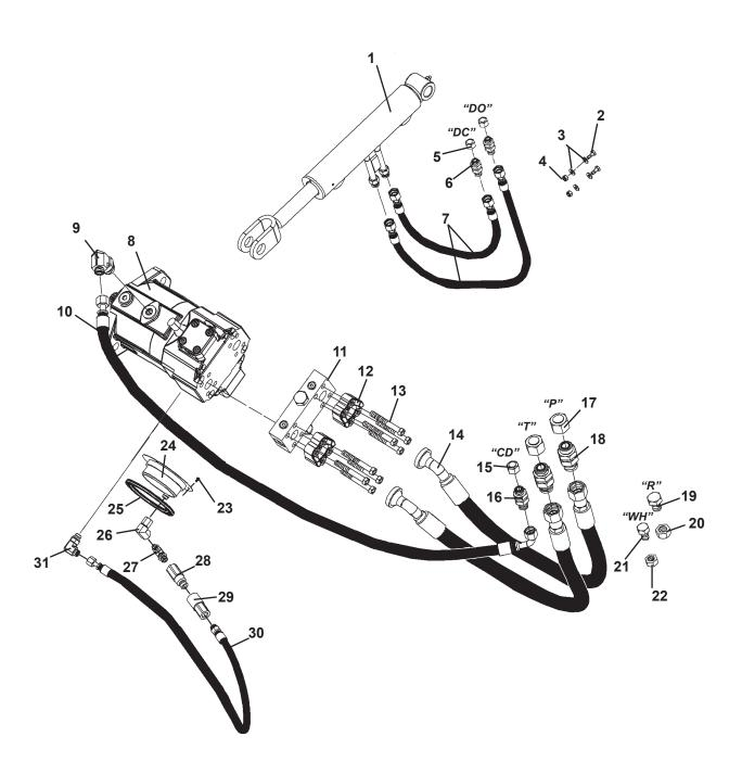
5-LINE - SKID STEER LOADER ASSEMBLY #115631 HYDRAULIC SYSTEM ASSEMBLY
