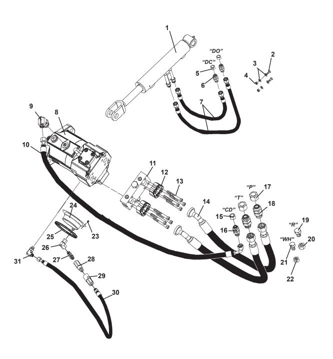
5-LINE - SKID STEER LOADER ASSEMBLY #115623 HYDRAULIC SYSTEM ASSEMBLY
