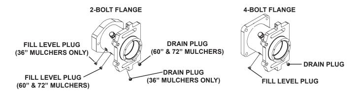
NOTICE: The Overhung Load Adapter assembly is a sealed system. If oil level is low, check all seals for damage.
