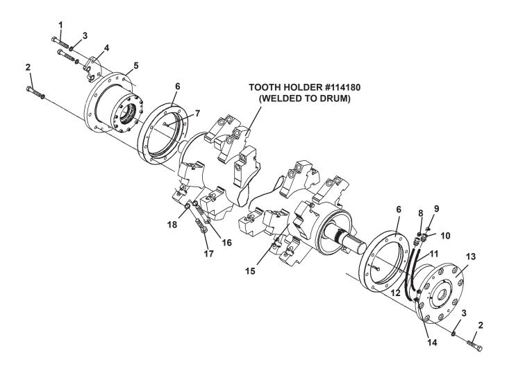
3-LINE COMBO (SKID STEER LOADER AND EXCAVATOR) ASSEMBLY - #115625 ROTOR ASSEMBLY
