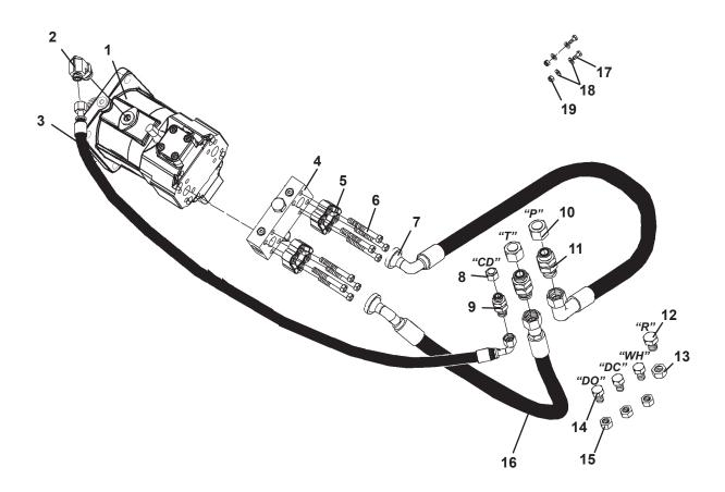
3-LINE - EXCAVATOR ASSEMBLY - #115624 HYDRAULIC SYSTEM ASSEMBLY
