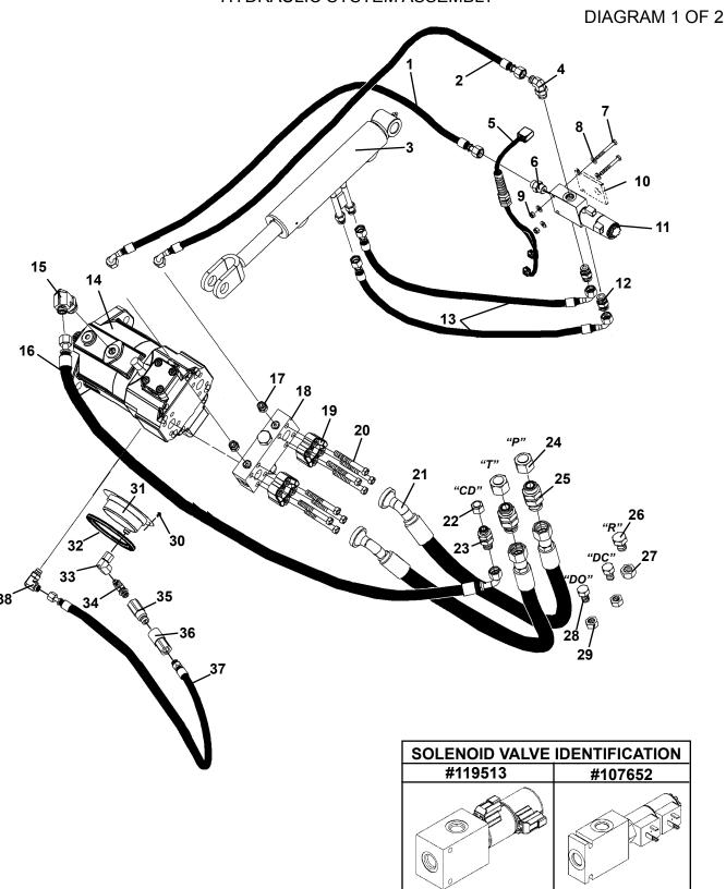
3-LINE - SKID STEER LOADER ASSEMBLY #115630 HYDRAULIC SYSTEM ASSEMBLY
