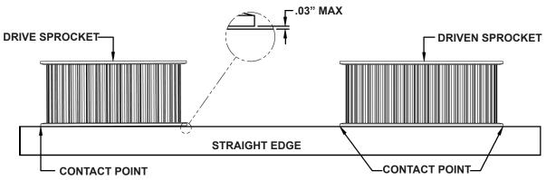
NOTICE: Failure to align the sprockets correctly will decrease the life of the belt.
