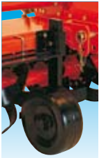
Front pair of wheels for working depth adjustment
