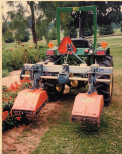
Model FP 66" frame with 2x12-16" tillage heads
