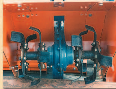
Detail of the blades, model FP. Hubs are easily added or removed to change head width.
